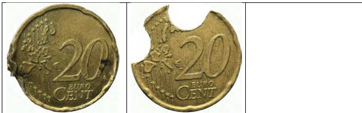
c. Bent and punched (due to impacts)
