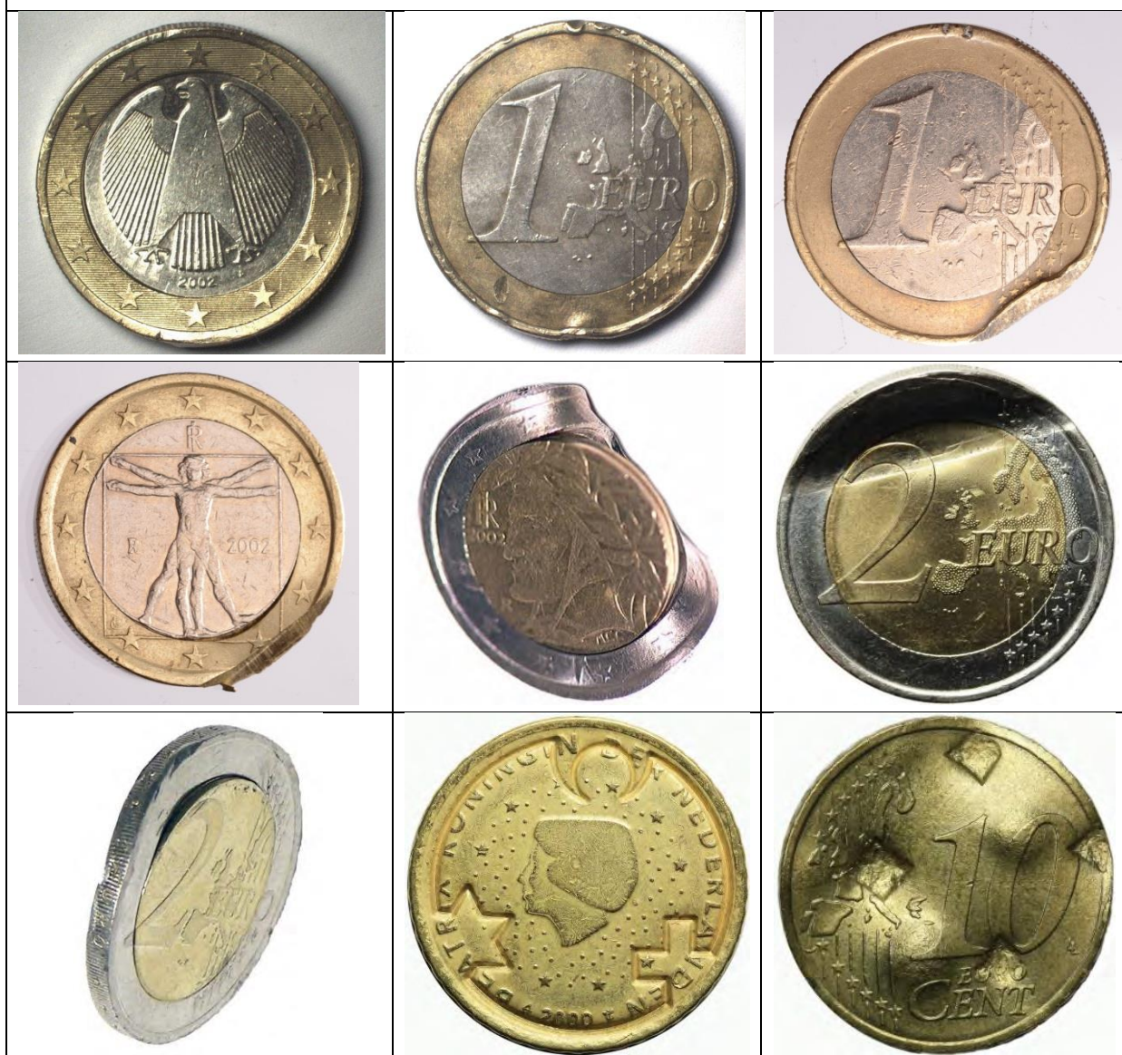
c. Bent and punched (due to impacts)
